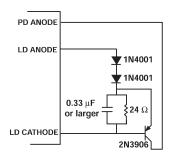
This circuit provides a fixed photodiode current. The 24  $\Omega$  resistor typically produces 30 mA of laser diode current. Vary the resistor size to change the current output.
