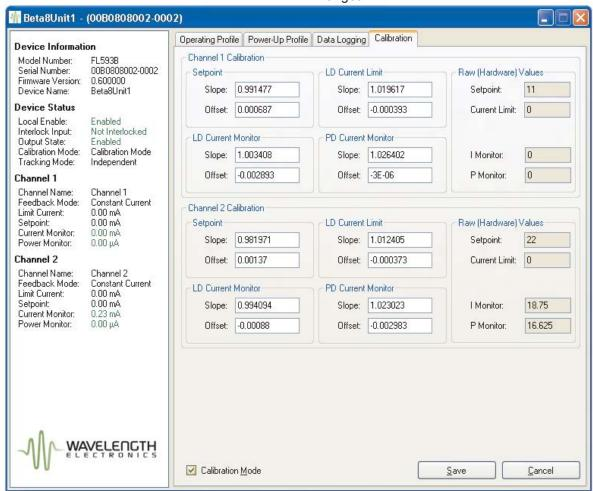
Figure 10: Calibration Tab
