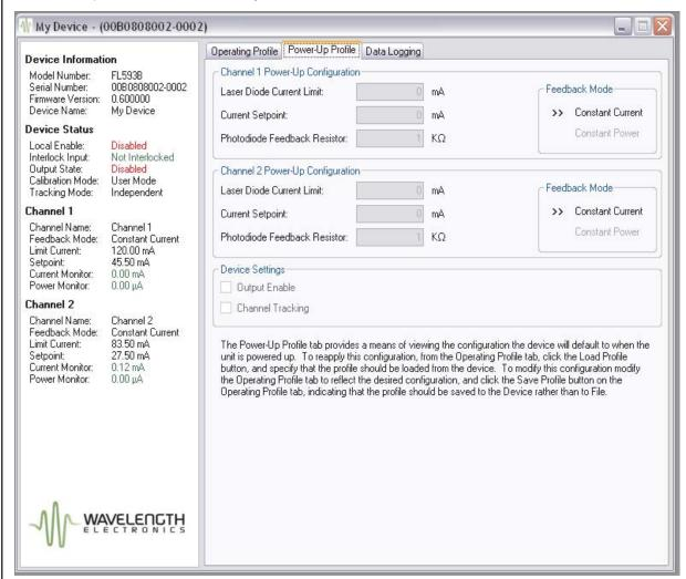
Figure 8: Power Up Profile Tab
